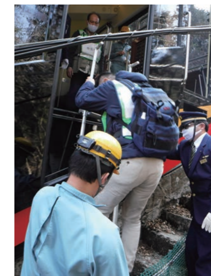
Guiding evacuation using emergency ladders from a cable car stopped between stations
